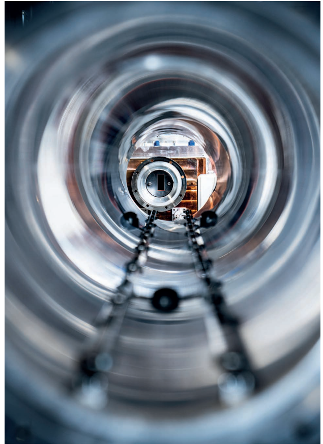
Interior view of a neutron guide that will transport and condition the neutron beam, designed and built at PSI with the support of Swiss industry. Photo: Artur G. Glavic, PSI
